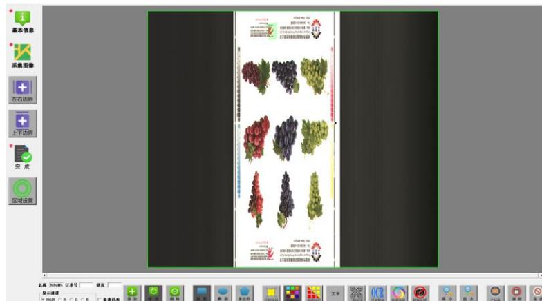
3). Sub-identification selection: the button operation is the same as 2), select a unique identification in the leftmost column image within a cycle of plate length (selection principle: unique, high image contrast)
